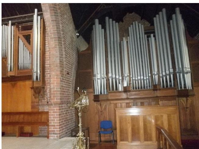
The organ has 3 manuals, 26 ranks and approximately 1850 pipes. It now has an electro-pneumatic action. At the time of rebuilding it was removed from the base of the tower and placed in the south transept where it remains.
